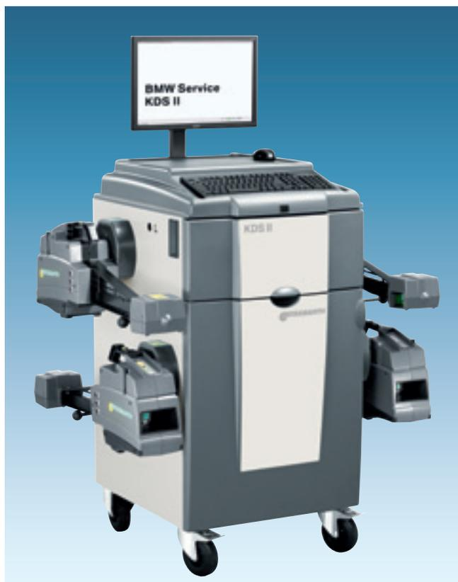
**The CCD camera technology developed by Beissbarth** is at the heart of the wheel alignment system. This is the third generation of KDS II featuring precision technology to perfection.
