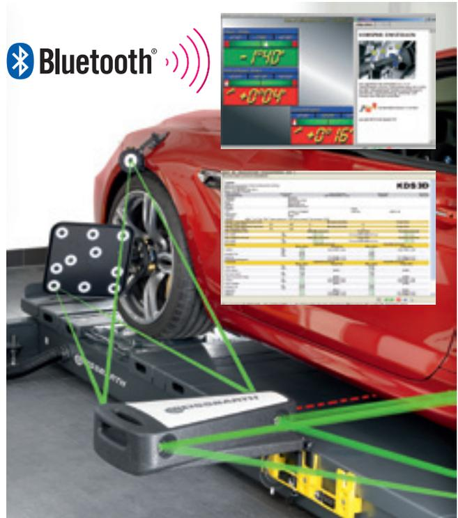
3D sensor heads and measurement boards in action
