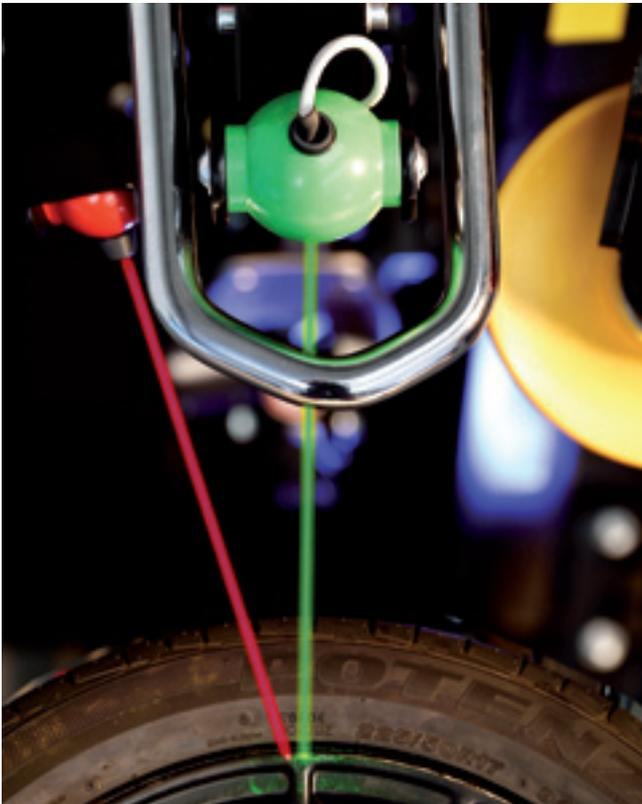
Two laser pointers determine the wheel size
