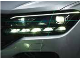
Cross laser: for the alignment to the centre of the headlight
