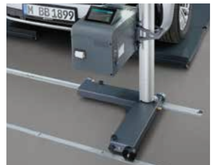
Rail system with MLD 9000
