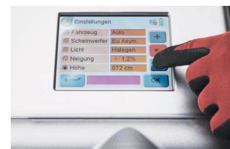
Operating panel can be rotated by 180° (operation with gloves is possible)
