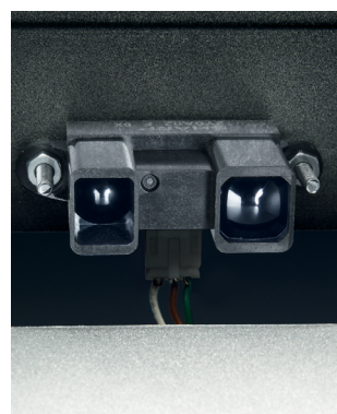
The height-measurement sensor automatically measures the installation height of the headlight (240 to 1450 mm) and shows the measured height on the display.
