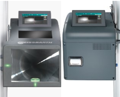
The operating panel is swivel-mounted into the light box. A single push allows the operator to switch the viewer direction – front for testing and back for for adjustment. The reading direction of the screen is switched simultaneously and automatically.
