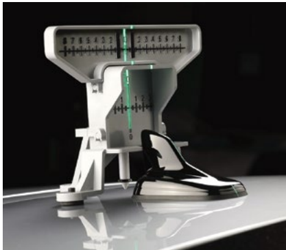
Positioning target for the roof antenna
