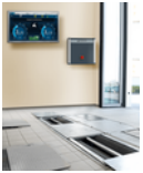
Car brake tester BD 4131 S10 | 2200mm | 3,7 kW | 230V |
