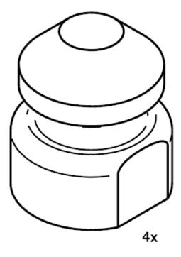
For space-saving storage of sensor heads when not in use
