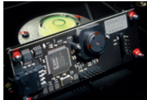
CMOS camera with high resolution and frame rate
